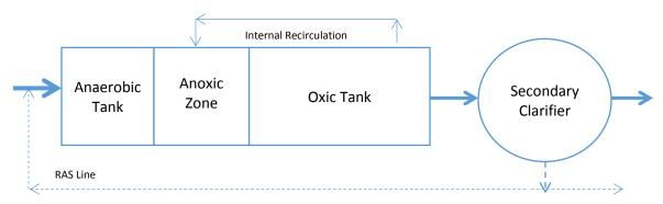
The Influent first enters Anaerobic Tank where phosphorus-accumulating bacteria release stored phosphorus to the wastewater. Ammonia passes through the anaerobic stage untreated. The underflow from secondary clarifier is recirculated to anaerobic tank to get mixed with fresh sewage by enhancing anaerobic conditions leading to removal of phosphorus biologically in absence of Oxygen.
